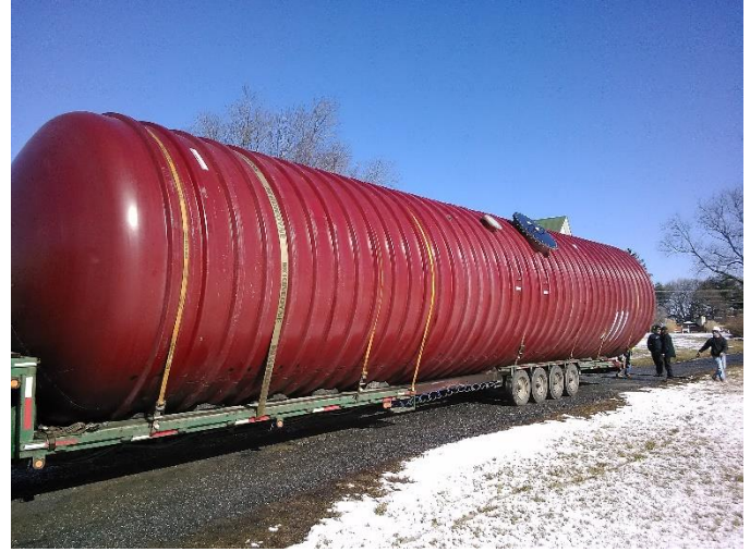
Ever wonder what a 42,000 gallon in-ground water tank looks like?
